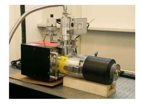
Source parameters Voltage range: 20 kV - 160 kV Target current range: 0 ~ 30 µA Spot size: 2 µm Target material: Titanium (4.5 keV) Fig. 13. a) Rigaku multilayer mirrors a) principle of work b) x-ray image of the beam
