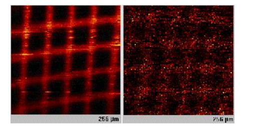
Fig. 8. Fluorescent image of the copper resolution grid imaged by the external beam a) 200 um distance from the exit window b) 1 mm distance
